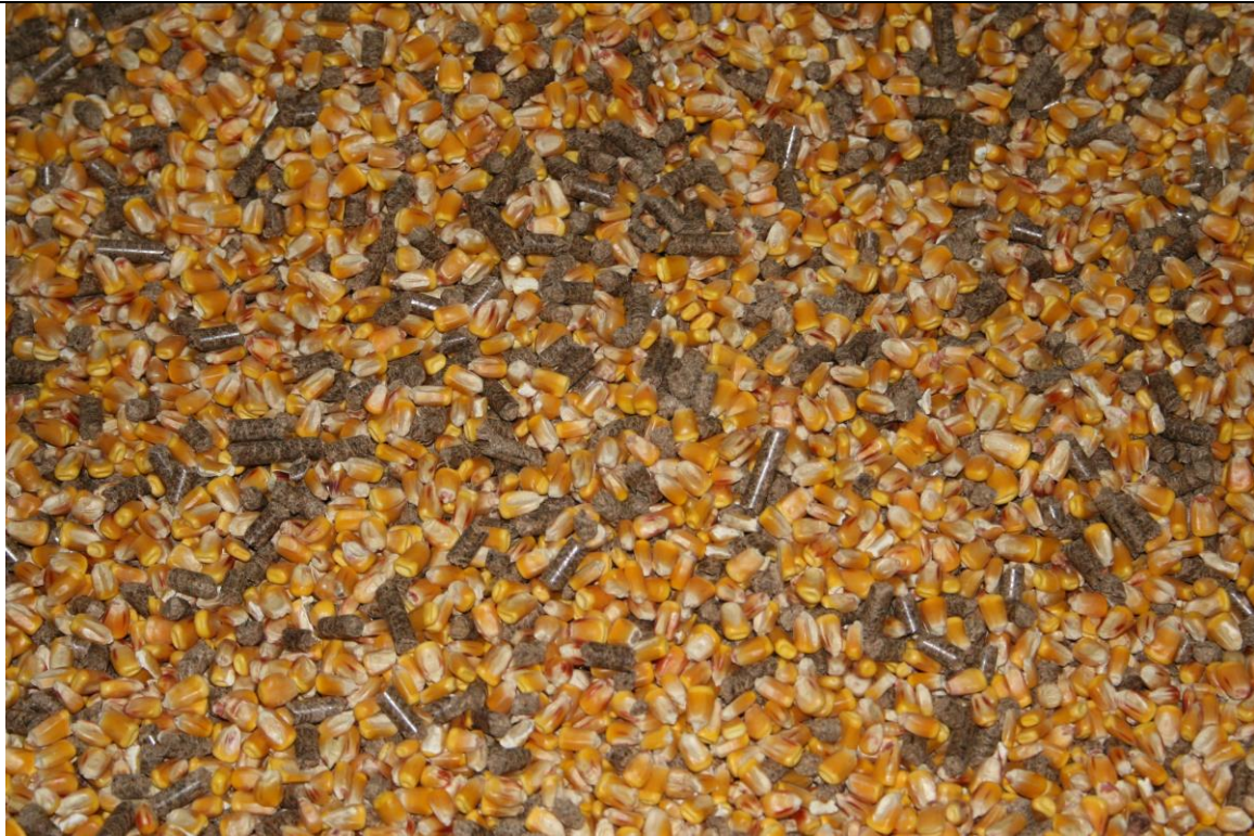
This is a photo of the 50/50 corn/pellet combination mix to fuel the stove.
